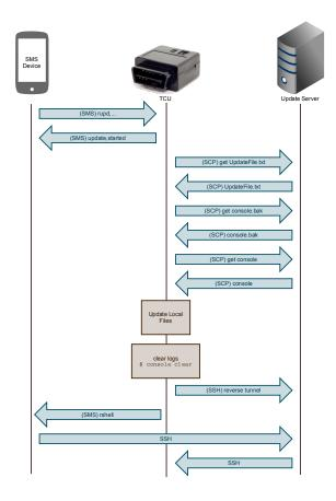
Figure 4: Remote exploitation via a malicious update server
